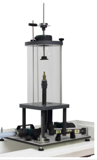
This equipment has been designed to verify the validity of the theoretical expressions that determine the force exerted by a jet on different types of blades.
